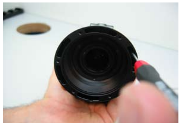
6) Remove 6 hex screws in side the slots.
