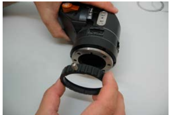
12) Screw the B4 clamp ring onto the mount and fix it with the one screw.
