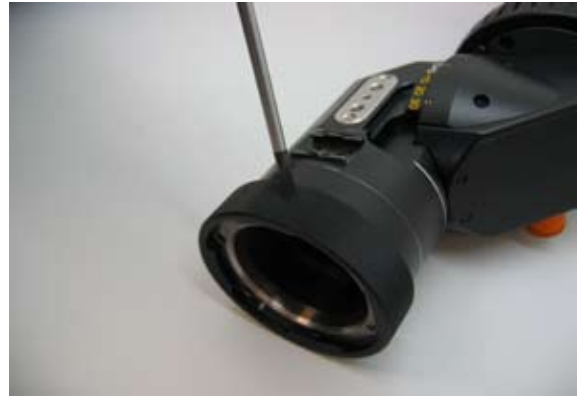
2) Release slotted adjustment screw at the side of the PL Mount clamp ring.
