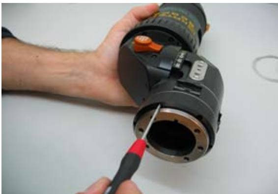
11) Fix 6 hex screws to hold the B4 mount in place.
