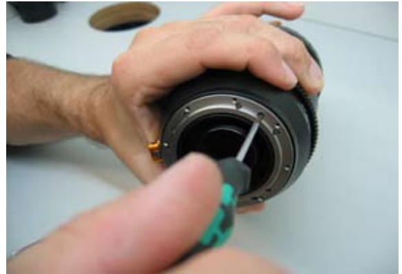
3) Remove 10 screws with hex screw driver.
