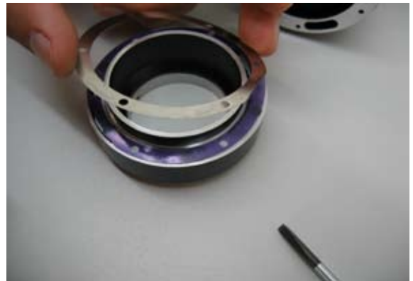
10) Carefully place the shims on the screw ends at the back side of the mount. Make sure the shims do not get squeezed or folded when adding the mount to the SKATER Scope.
