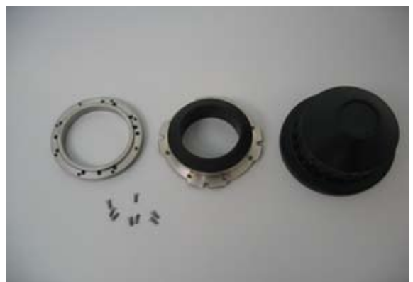
7) Keep the metal adapter ring, PL Mount, Cap and 8 screws in a safe place until you want to change it back to PL mount version.
