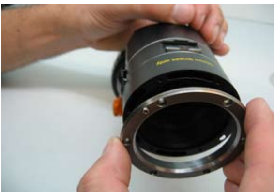
5) Carefully remove the metal mount ring.
