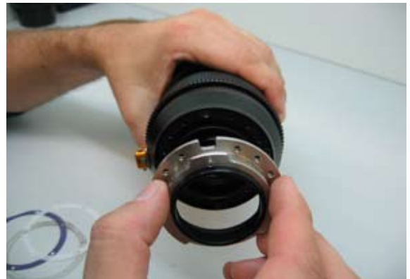
5) Replace with B4 Mount and carefully add delivered shims. Lined up the pin on the mount with the middle of the SKATER Scope logo.
