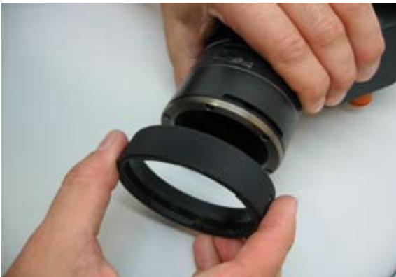
3) Turn the clamp ring until it comes off the mount.
