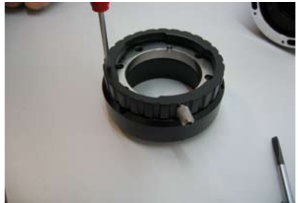
8) Prepare the B4 Mount by releasing the adjustment screw. Remove the clamp ring from the mount.
