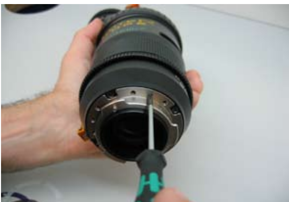
6) Fix with 10 slotted screws.
